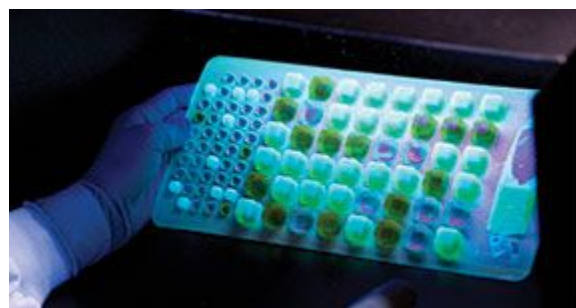
Figure 3. IDEXX Quanti-Tray under 365nm UV light, the presence of E. coli indicated by fluorescing wells.
